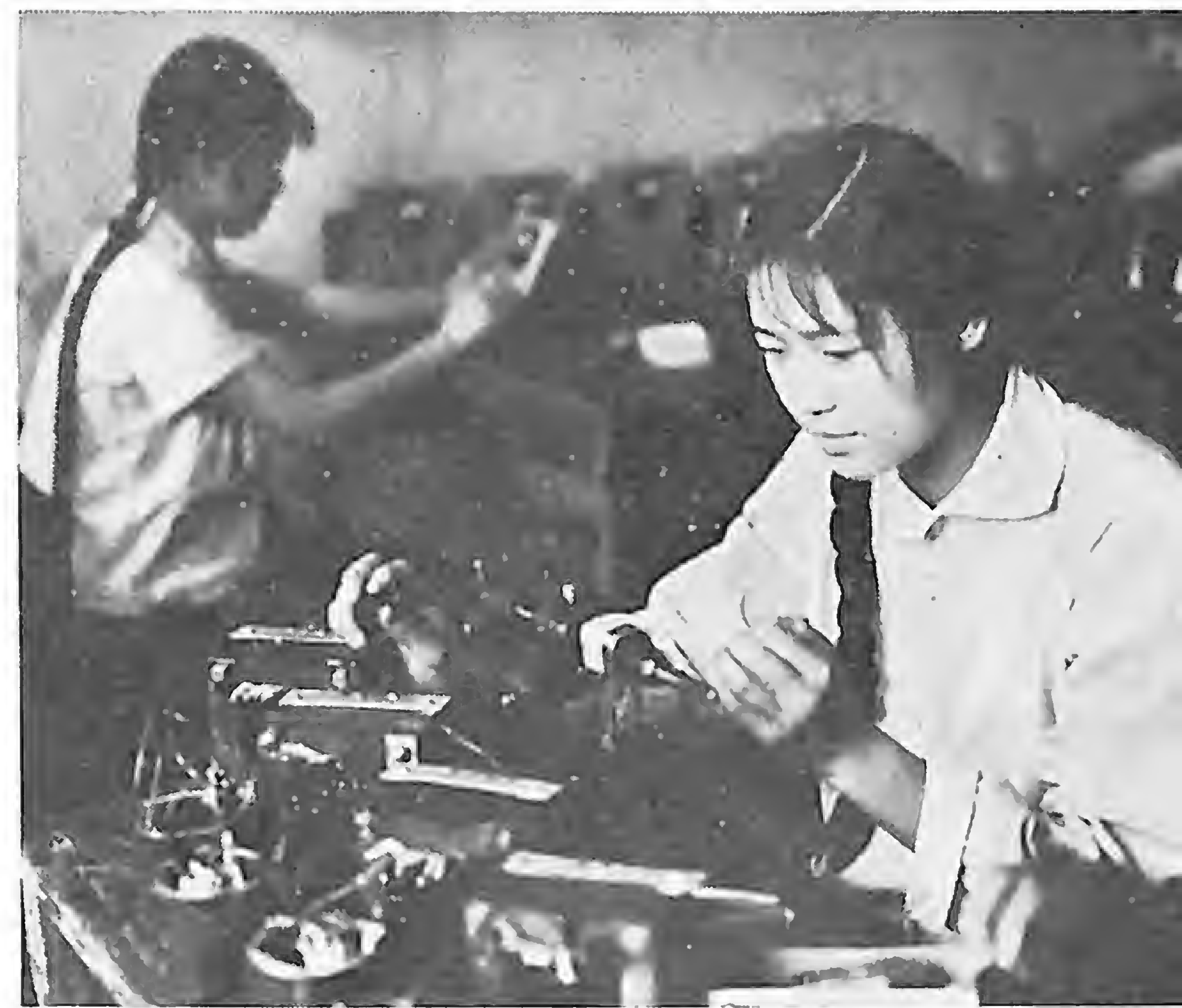
A student winds a coil in the school-run power-supply shop.
